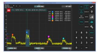
Set up to 10 *MARKERS* for input level measurements. *POWER IN BAND* menu allows measuring input power for desired bandwidth (BW).
