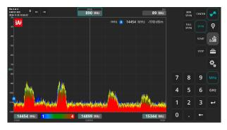
Visual representation of multiple spectrum curves overlap in heat map format
