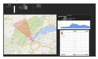
Allows synchronizing GPS coordinates from external logger with saved spectrum curves. Displays information such as spectrum curves, elevation and location on the map. Supports KML file export.
